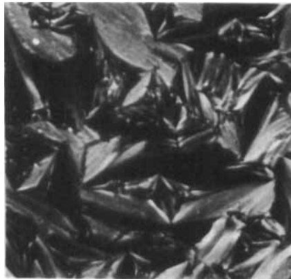
FIGURE III Mixture with 15\text{ mol } \% CN : focal conic texture with large monodomains.
