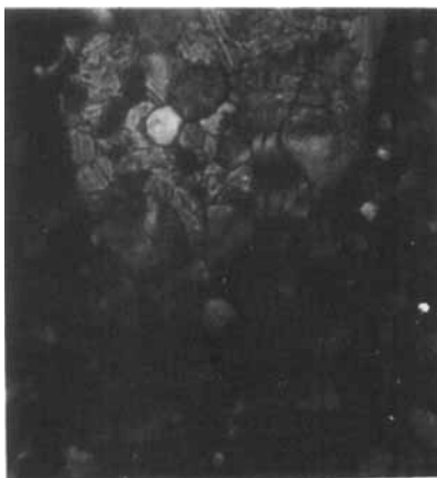
FIGURE I a Mixture with 85 mol % CN : platelets texture.
